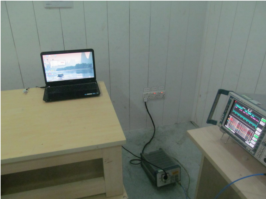
FCC RADIATED EMISSION TEST SETUP
