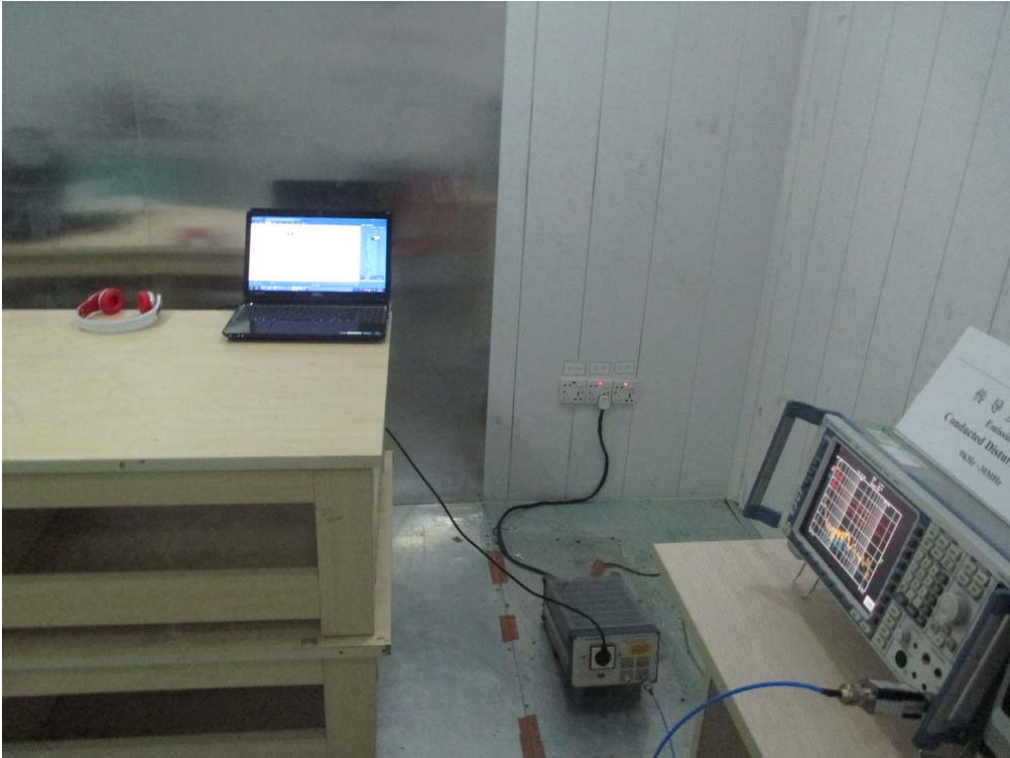
FCC RADIATED EMISSION TEST SETUP
