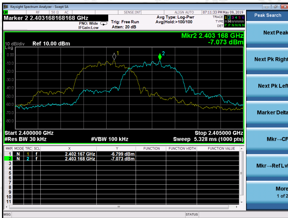
TEST PLOT FOR FREQUENCY SEPARATION
