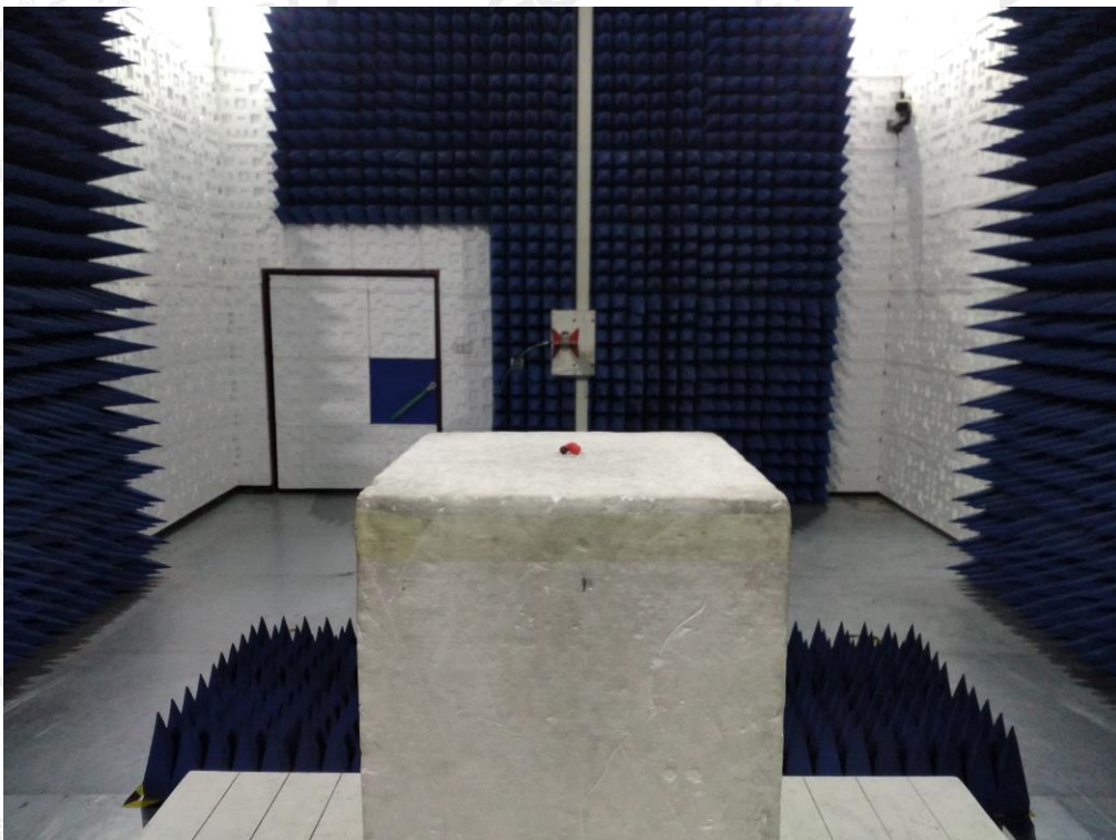
RADIATED EMISSION TEST SETUP ABOVE 1GHZ
