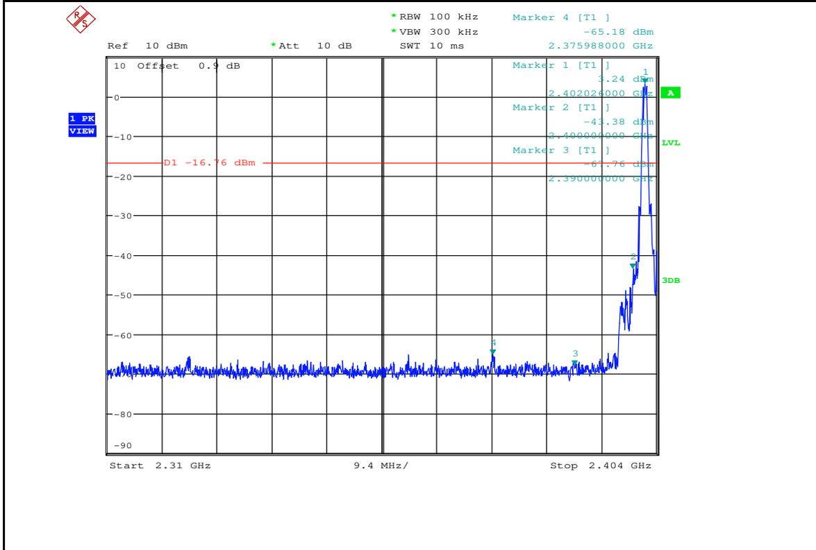
Band-edge for RF Conducted Emissions\_BLE\_2480\_Ant1
