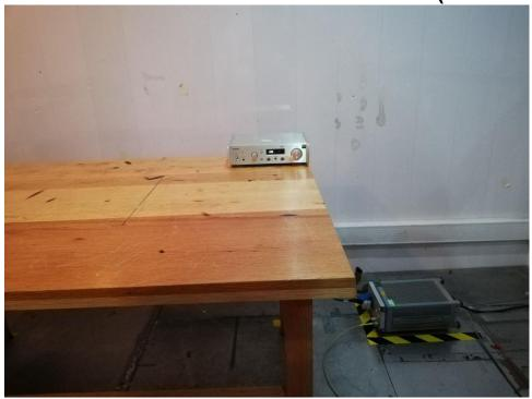
1.2 Radiated Spurious Emissions Test Setup
