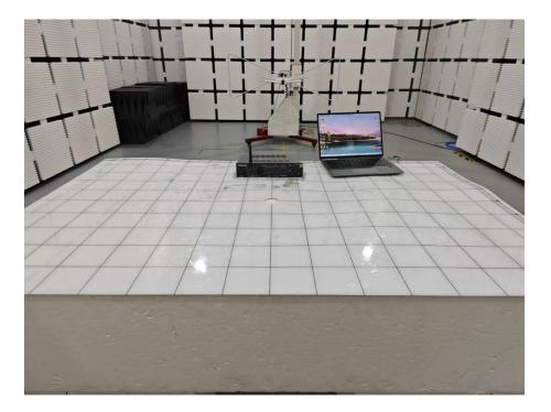
Set-up for Radiated Spurious Emission, Below 1GHz
