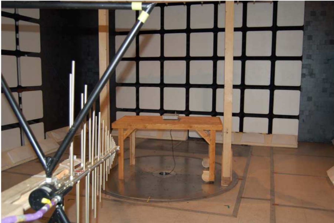
FCC Part 15.109 and RSS 210 - Radiated Emissions 30 MHz – 1GHz
