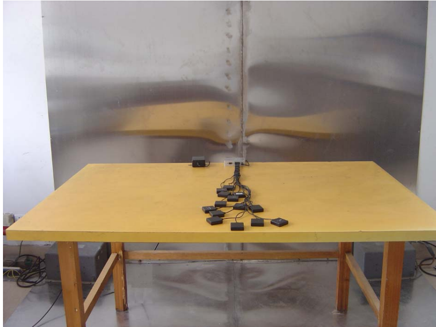
Conducted Emissions - Front View (Charging Mode)
