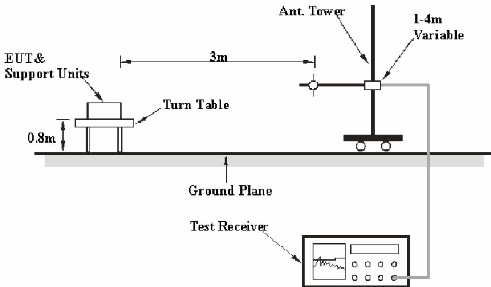
The radiated emission and out of band emission tests were performed in the 3 meters chamber B, using the setup accordance with the ANSI C63.4-2003. The specification used was the FCC 15.209, FCC 15.249 and FCC 15.109 limits.
