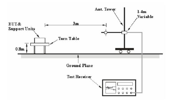
The radiated emission and out of band emission tests were performed in the 3 meters chamber B, using the setup accordance with the ANSI C63.4-2003. The specification used was the FCC 15.209, FCC 15.249 and FCC 15.109 limits.
