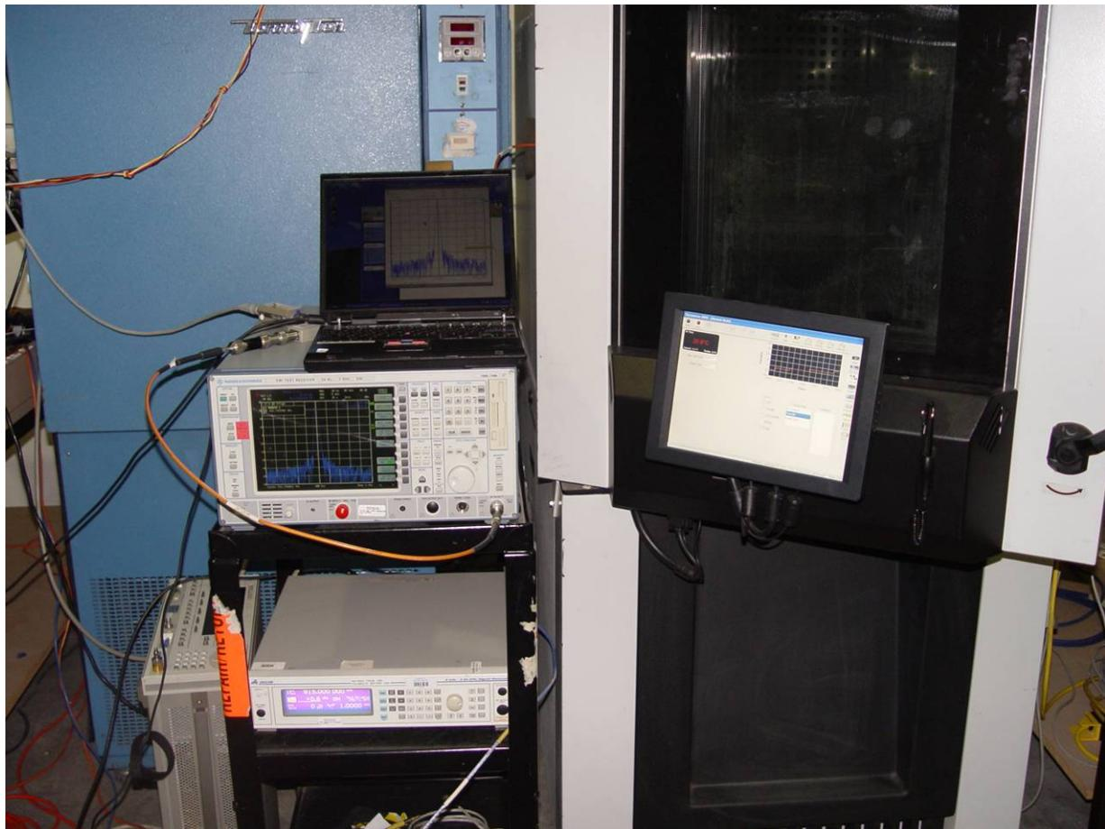
Frequency Error Test Set-Up – Environmental Chamber
