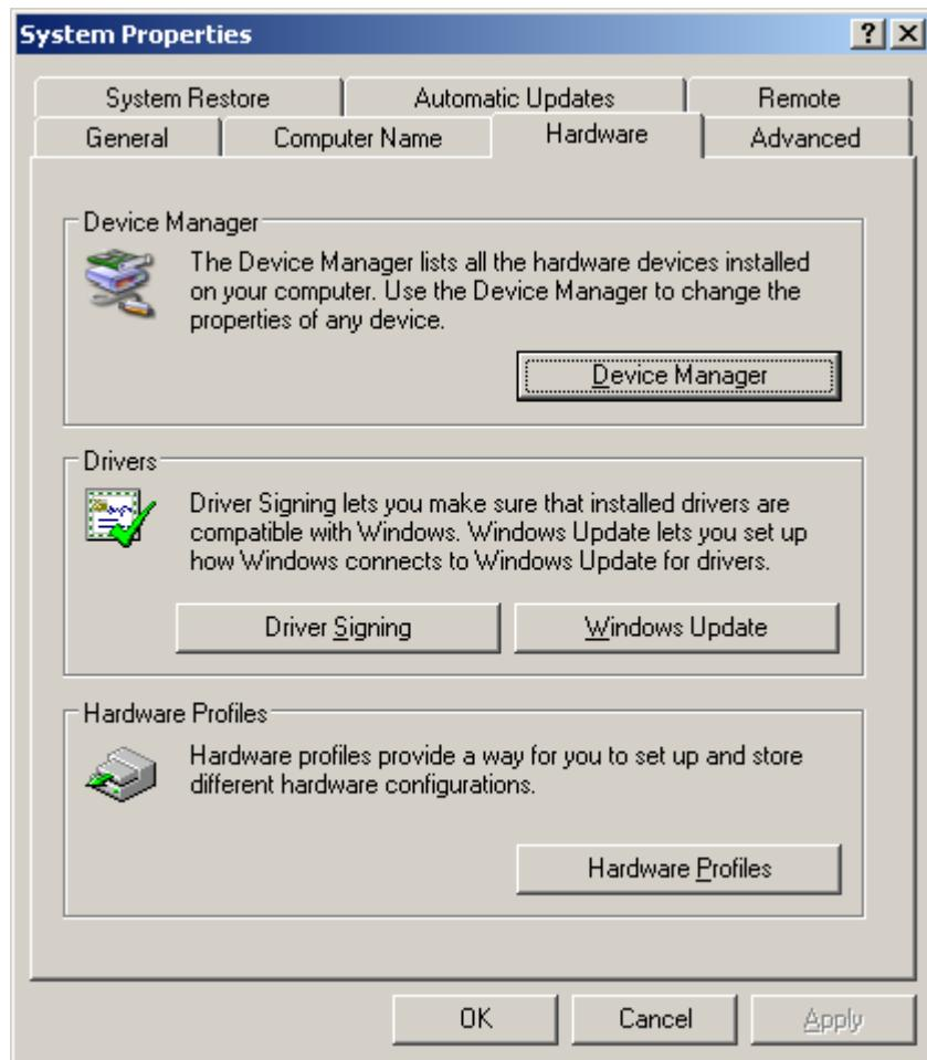
Click "Device Manager" and expand the "Ports (Com and LPT)" option. Look for the *Thinkify USB-Serial Bridge* entry and note the com port.
