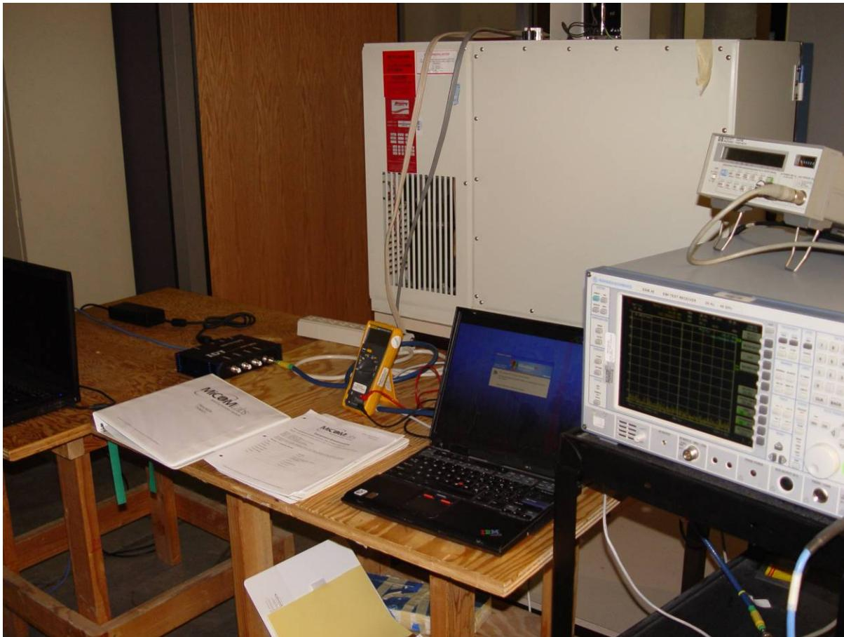
***Frequency Error Test Set-Up – Environmental Chamber***
