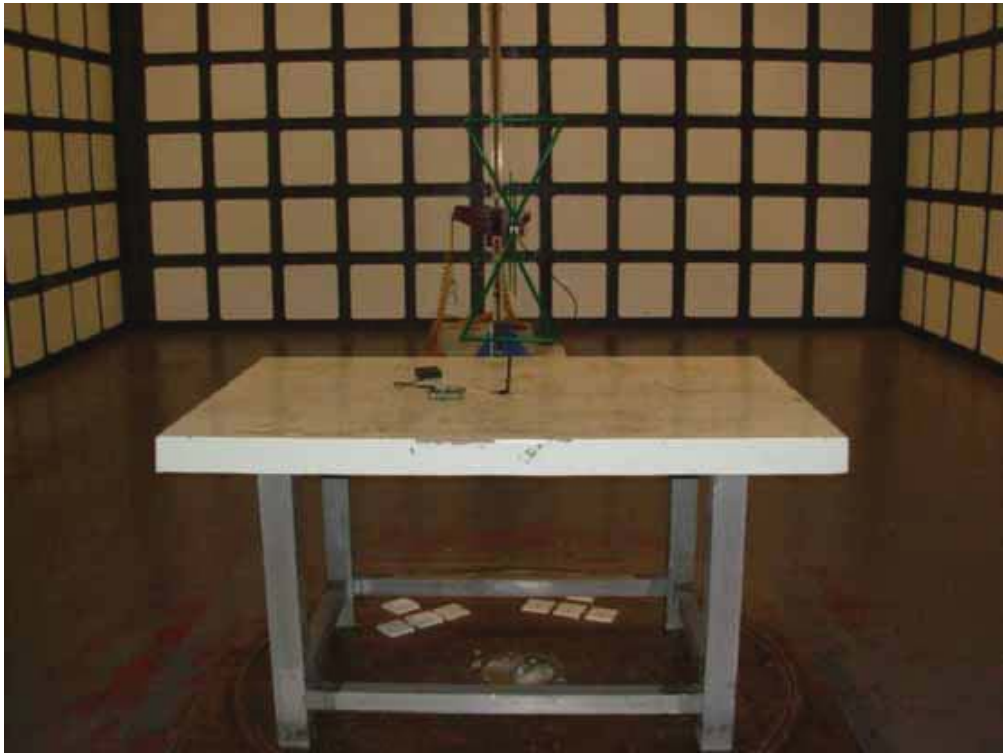
FRONT VIEW OF RADIATED EMISSION TEST (BELOW 1GHz)(ANTENNA 2)
