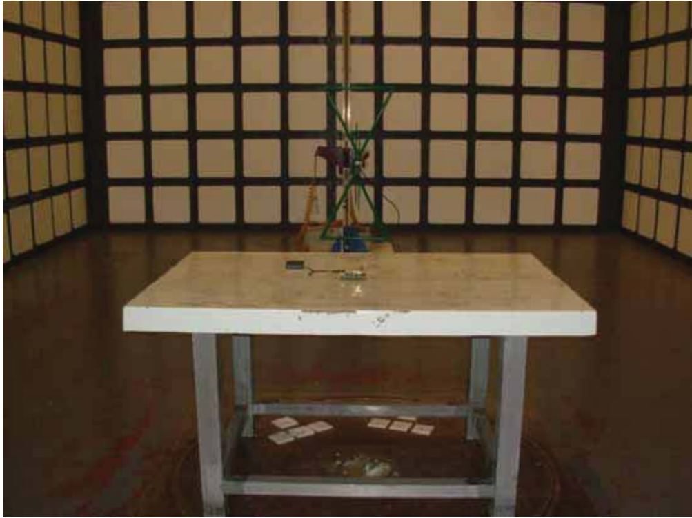
FRONT VIEW OF RADIATED EMISSION TEST (BELOW 1GHz)(ANTENNA 1)
