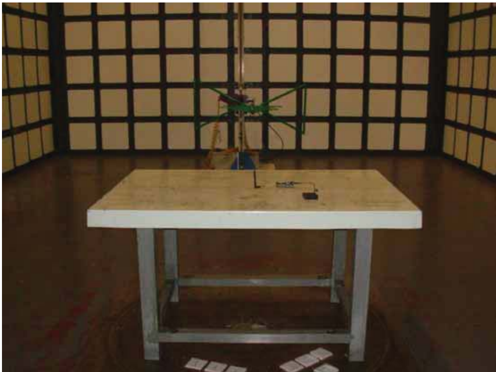
BACK VIEW OF RADIATED EMISSION TEST (BELOW 1GHz)(ANTENNA 2)
