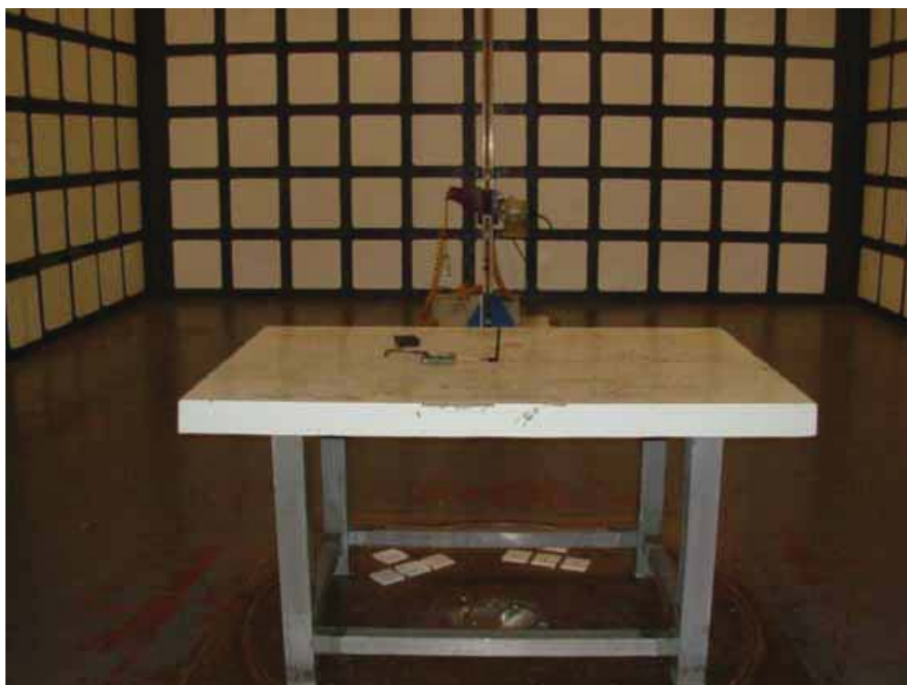
FRONT VIEW OF RADIATED EMISSION TEST (ABOVE 1GHz)(ANTENNA 2)
