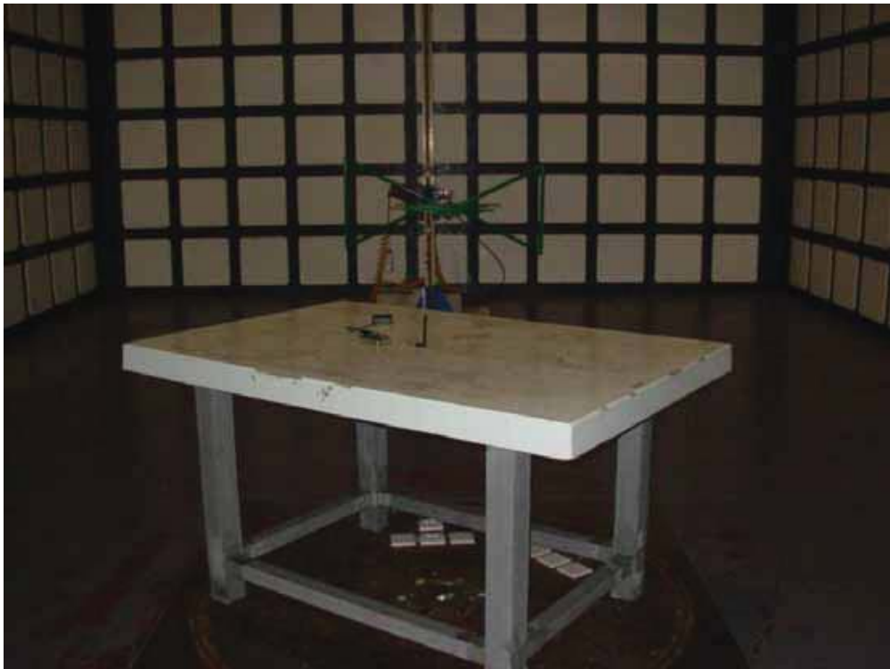
SETUP WITH MAXIMUM DETECTED EMISSION AT HORIZONTAL POLARIZATION (TRANSMITTING ANTENNA2 CH26)
