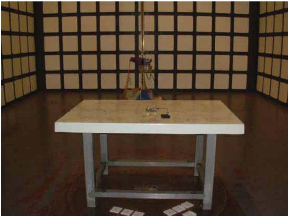
BACK VIEW OF RADIATED EMISSION TEST (ABOVE 1GHZ)(ANTENNA 1)
