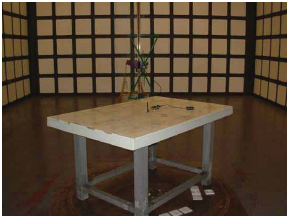
SETUP WITH MAXIMUM DETECTED EMISSION AT VERTICAL POLARIZATION (TRANSMITTING ANTENNA2 CH26)
