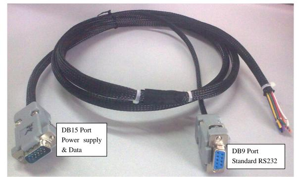
To make user connect the device easily, there is a set of cable provided with the device. One side of the cable connects "Power & Data" port of the device. Thereare two types of signal at the other side, power parts and RS-232 femaleconnector.
