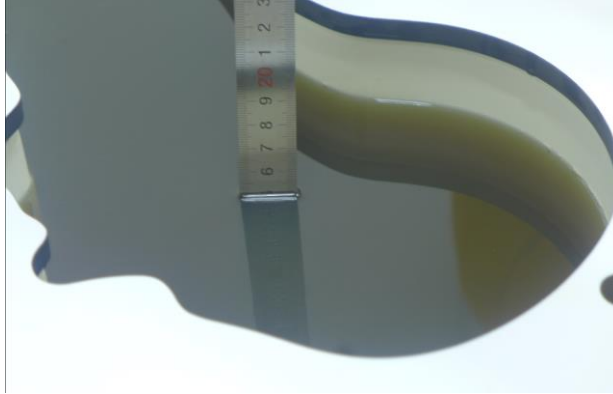
Photo 1: Tissue Simulant Liquid for HBBL600-10000MHz
