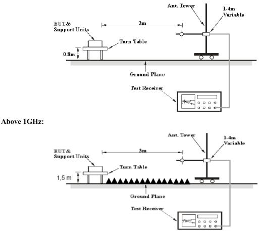
The radiated emissions were performed in the 3 meters distance, using the setup accordance with the ANSI C63.10-2013. The specification used was the FCC 15.209, and FCC 15.247 limits.
