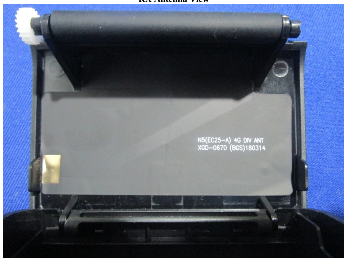
RX Antenna View
