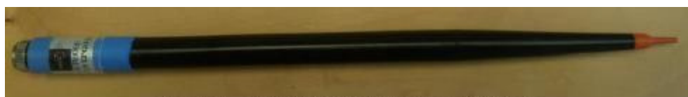
Figure 1 – MVG COMOSAR Dosimetric E field Dipole
