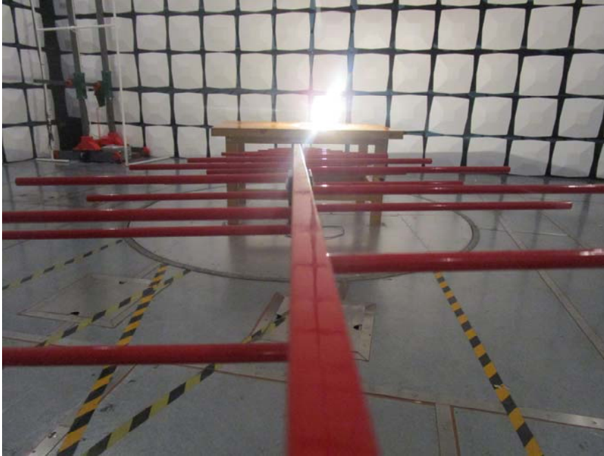
Radiated Emission View (Below 1GHz)
