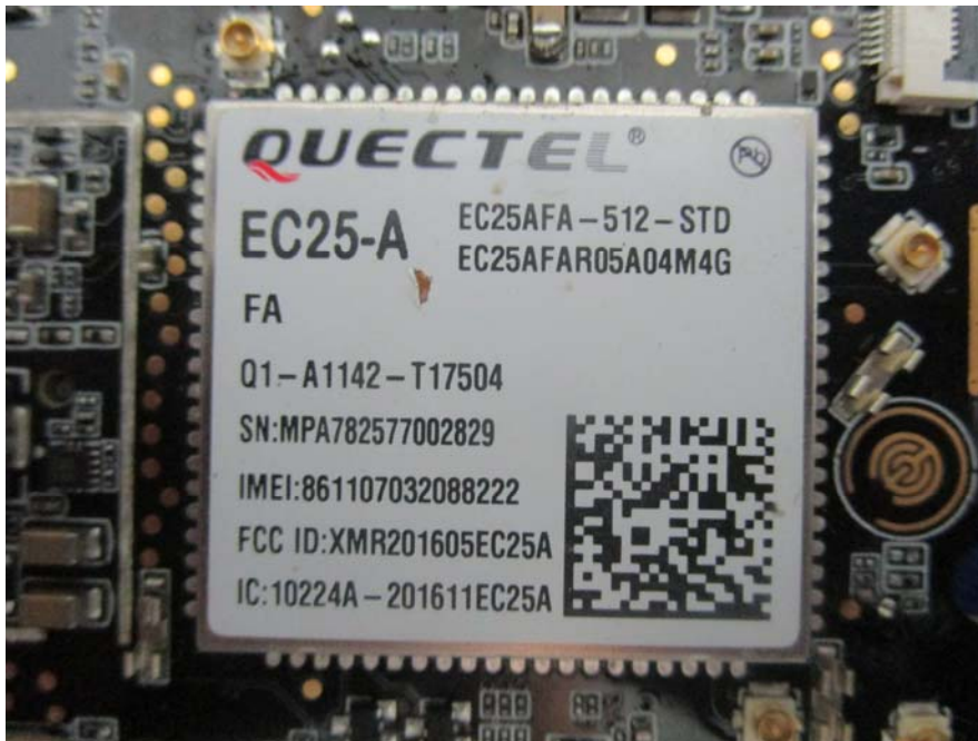
EUT –RF Module View
