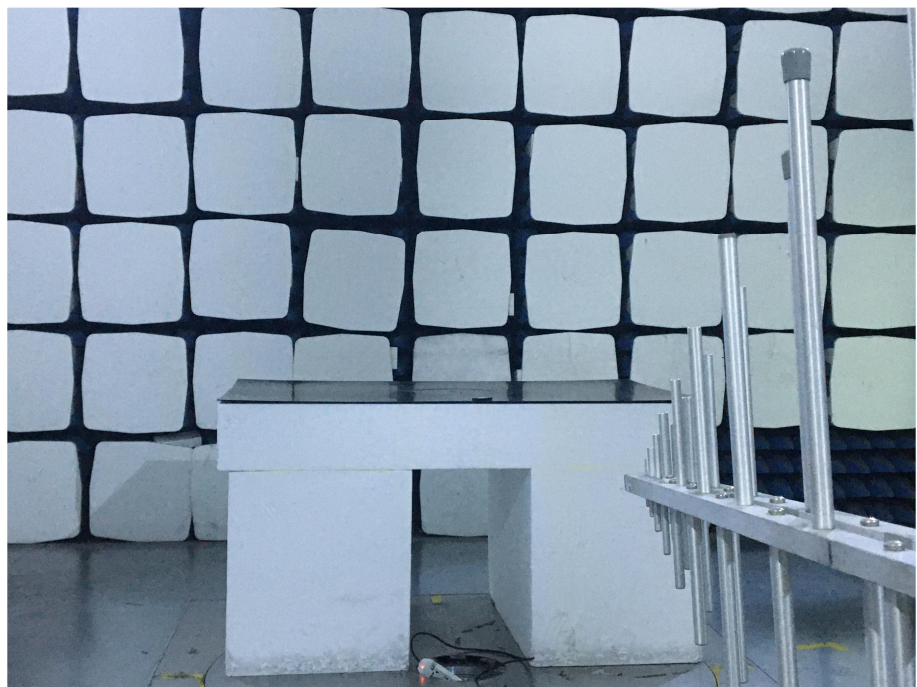
Radiation Emission Test Setup (30MHz to 1GHz)
