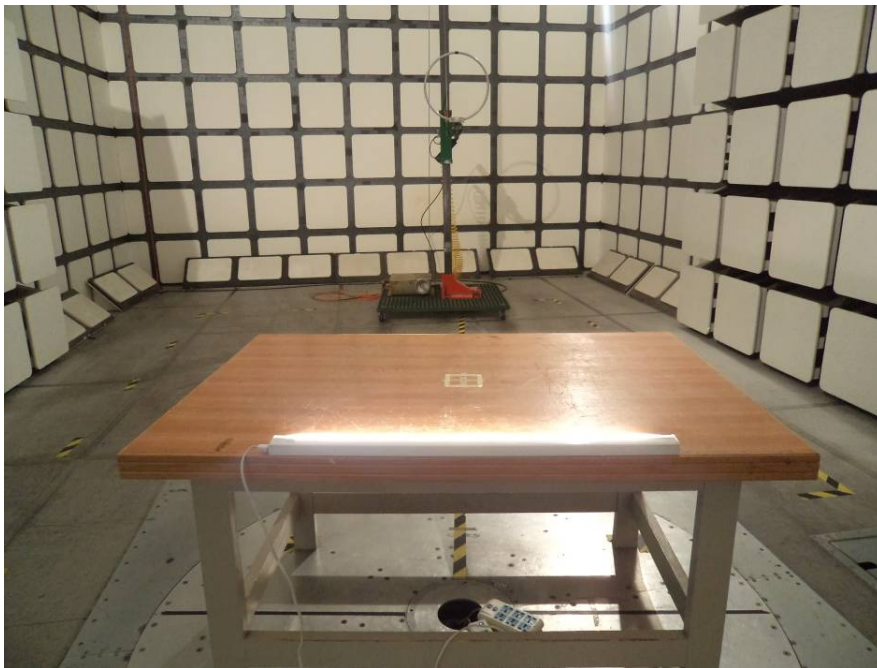
Radiated Emissions – Rear View
