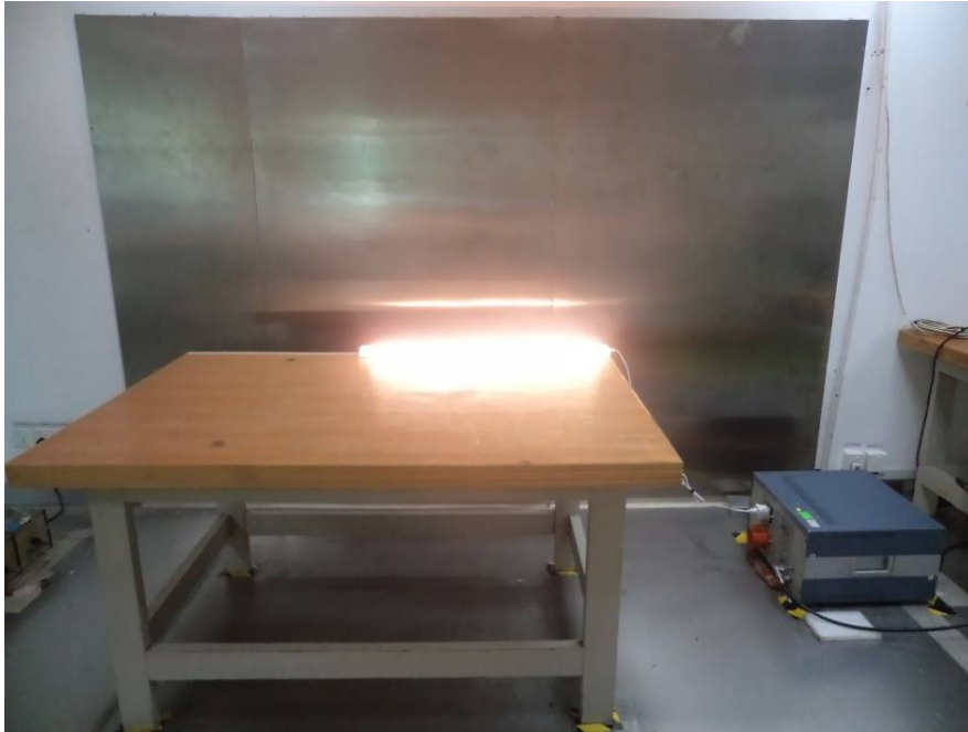
AC Line Conduction Emissions – Front View
