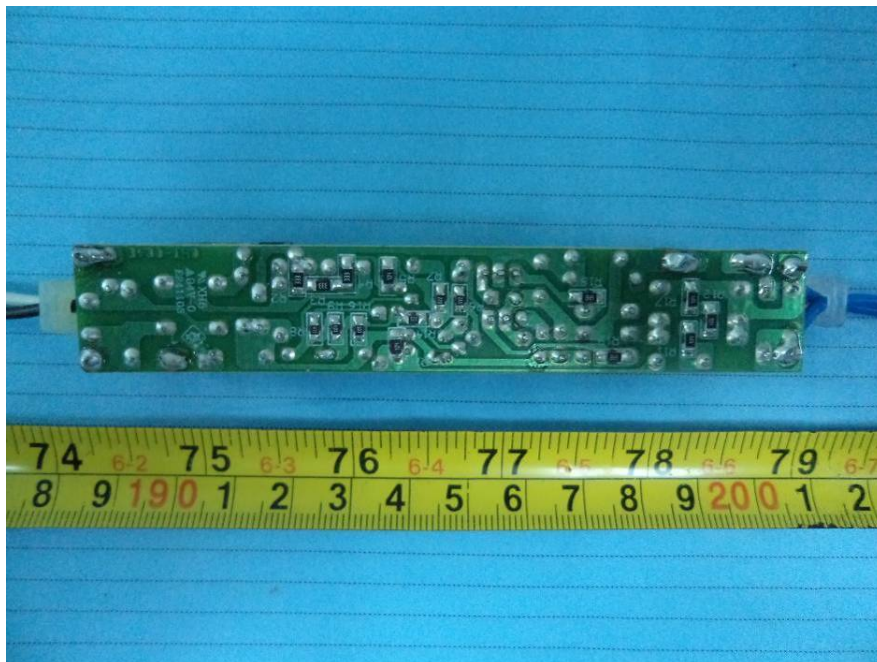
EUT – Electronic Ballast Main Board Bottom View
