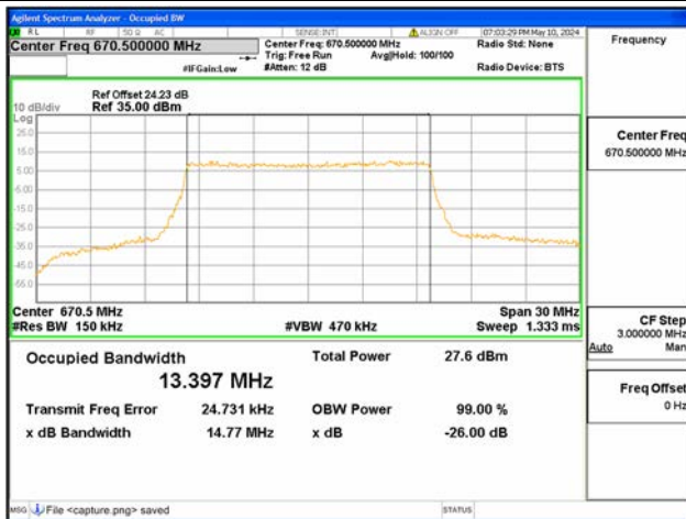
B71 / 15MHz / 64QAM/ Low CH
