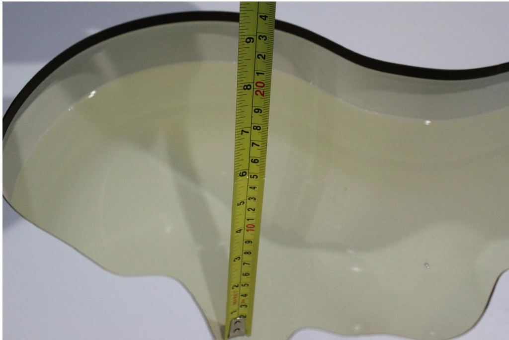
Picture 7-7: Liquid depth in the Head Phantom(5GHz)
