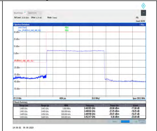
1-N77-3450-3550-PC2-30-90-L-3-DFT-PI2BPSK-Outer_Full-240@0-Ant5-1--PASS-see graph
