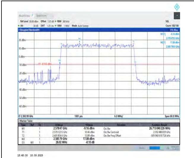
1-N41-PC2-30-30-M-2-DFT-PI2BPSK-Outer_Full-75 @0-Ant3-26.713-28.020-≤30-PASS
