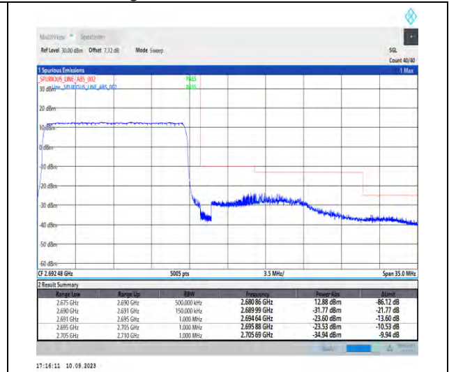
1-N41-PC2-30-15-H-3-DFT-PI2BPSK-Outer_Full-3 6@0-Ant3-1--PASS-see graph
