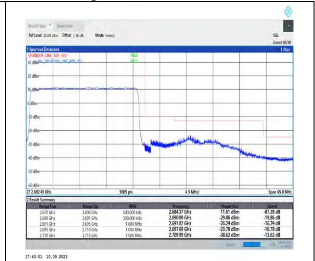
1-N41-PC2-30-20-H-3-DFT-PI2BPSK-Outer_Full-5 0@0-Ant3-1--PASS-see graph
