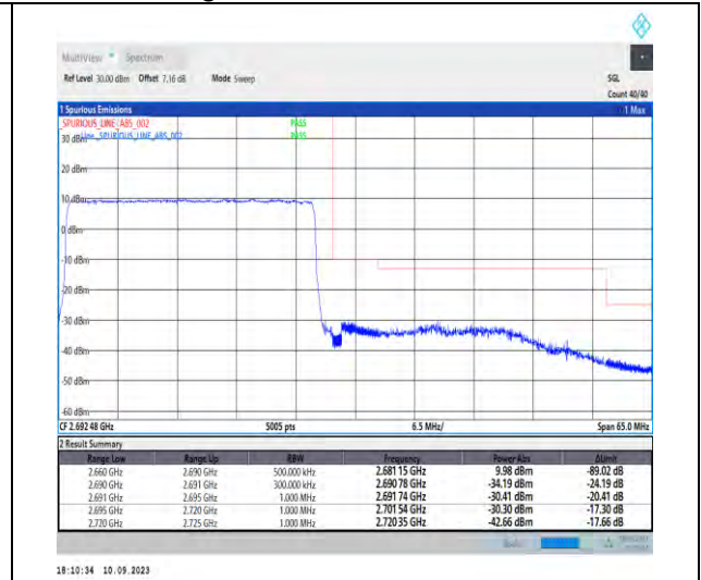
1-N41-PC2-30-30-H-3-DFT-PI2BPSK-Outer_Full-7 5@0-Ant3-1--PASS-see graph
