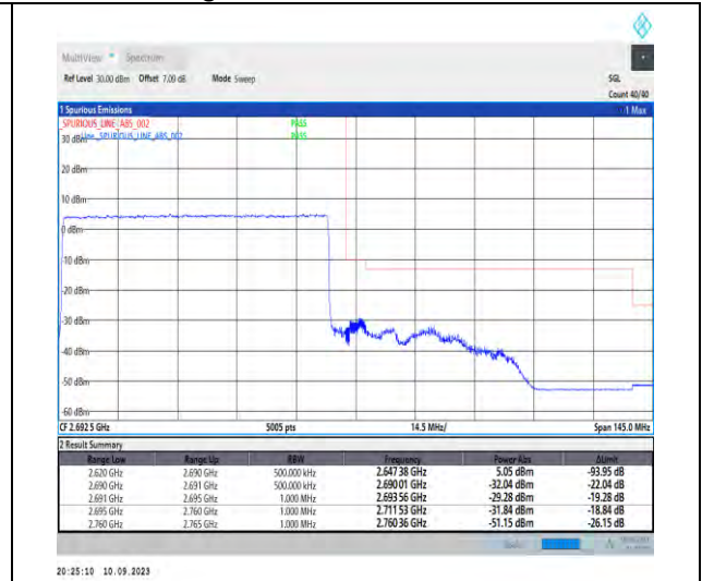
1-N41-PC2-30-70-H-3-DFT-PI2BPSK-Outer_Full-1 80@0-Ant3-1--PASS-see graph
