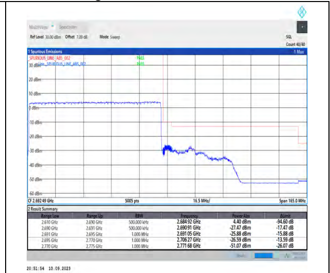
1-N41-PC2-30-80-H-3-DFT-PI2BPSK-Outer_Full-2 16@0-Ant3-1--PASS-see graph
