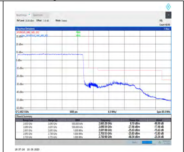
1-N41-PC2-30-40-H-3-DFT-PI2BPSK-Outer_Full-1 00@0-Ant3-1--PASS-see graph
