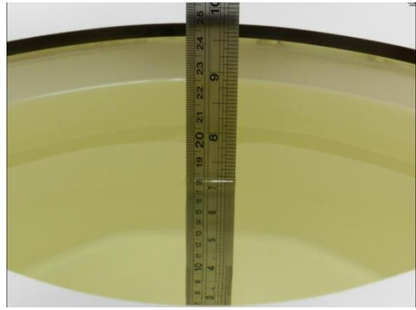
Fig 11.2 Photo of Liquid Height for Body SAR
