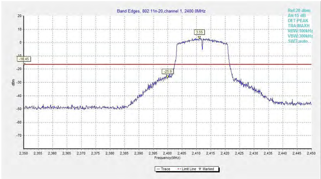
Fig.A.5.5 Band Edges (802.11n-HT20, Ch 1)
