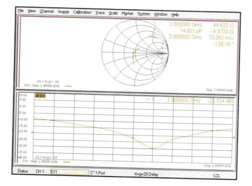
Impedance Measurement Plot for Body TSL
