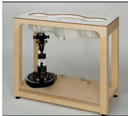
Picture C.10: SAM Twin Phantom
