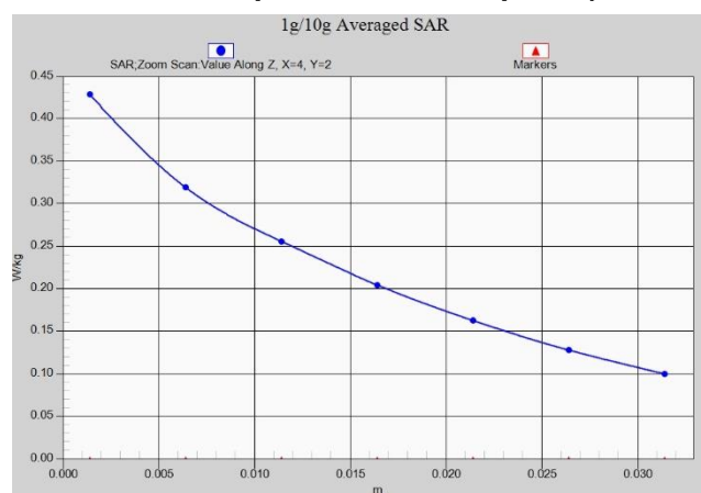
Fig. 1-14 Z-Scan at power reference point (CDMA BC0)
