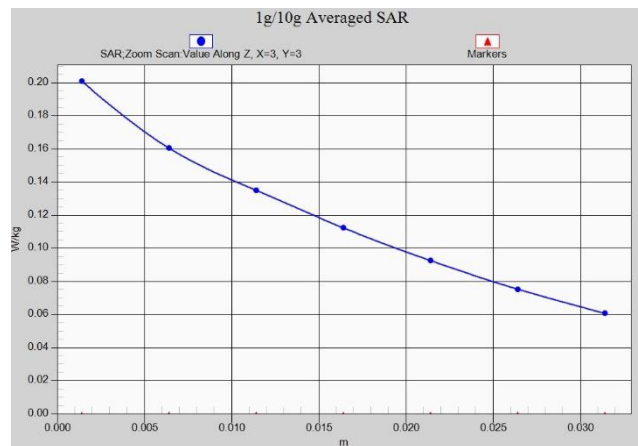
Fig. 1-39 Z-Scan at power reference point (LTE Band71)
