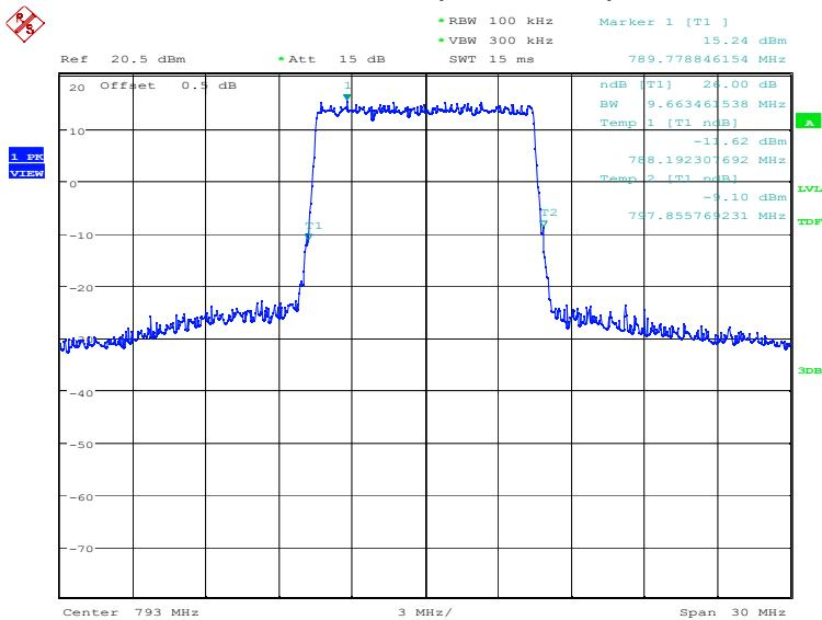
**LTE band 14, 10MHz Bandwidth,16QAM (-26dBc BW)**
