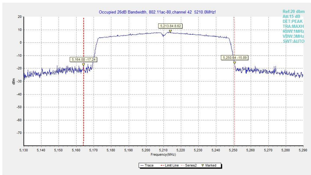
Fig.29 Occupied 26dB Bandwidth (802. 11ac-HT80, 5210MHz)
