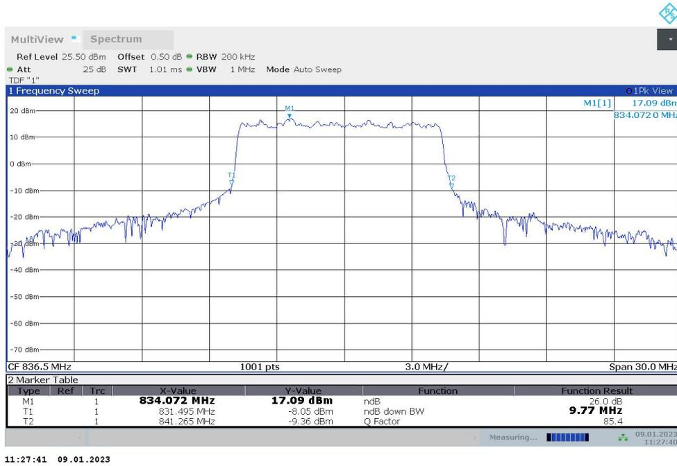
**n5,10MHz Bandwidth,DFT-s-QPSK (-26dBc BW)**
