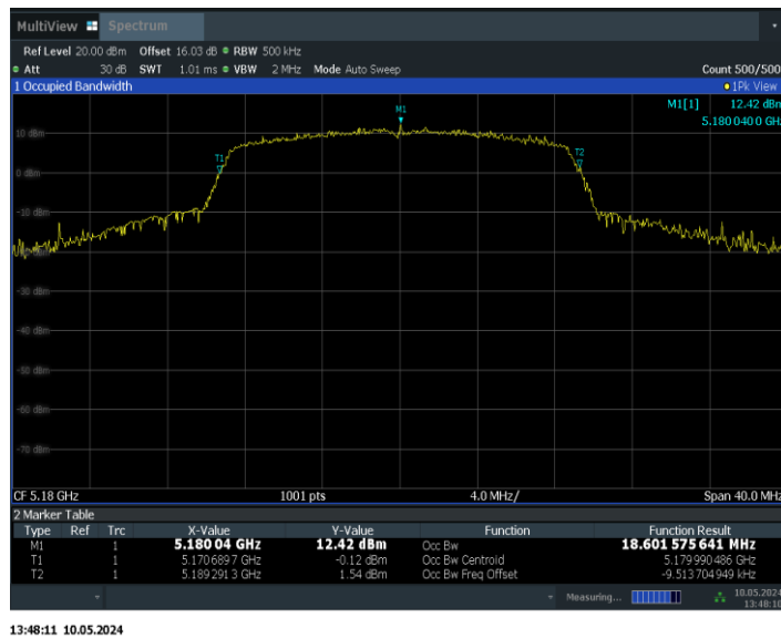
Fig.31 99% Occupied bandwidth (802.11n-HT20, 5180MHz)
