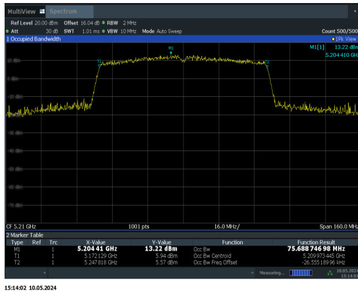
Fig.36 99% Occupied bandwidth (802.11ac-VHT80, 5210MHz)
