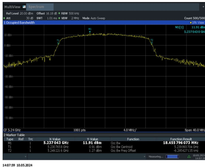
Fig.33 99% Occupied bandwidth (802.11n-HT20, 5240MHz)
