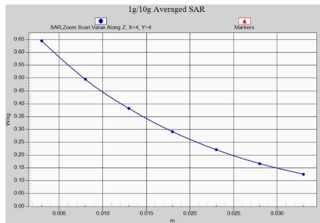
Fig. 1-15 Z-Scan at power reference point (CDMA BC0)
