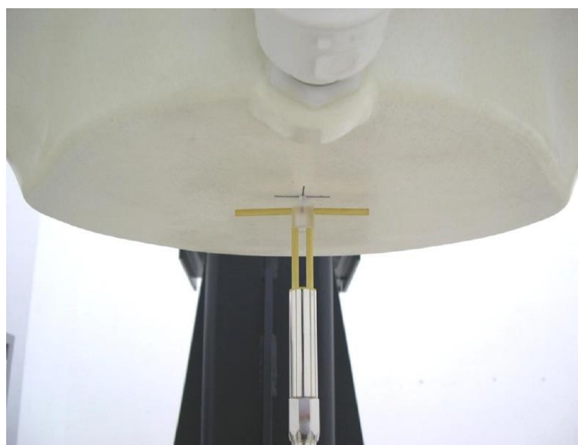
Picture 8.2 Photo of Dipole Setup
