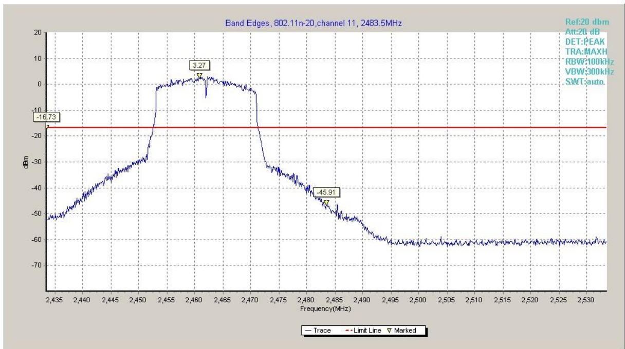
Fig.A.5.1.6 Band Edges (802.11n-HT20, Ch 11)
