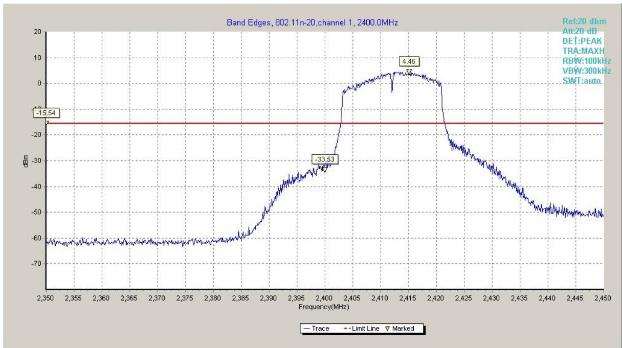
Fig.A.5.1.5 Band Edges (802.11n-HT20, Ch 1)
