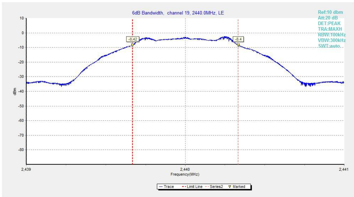
Fig.23. 6dB Bandwidth: GFSK, 2440 MHz
