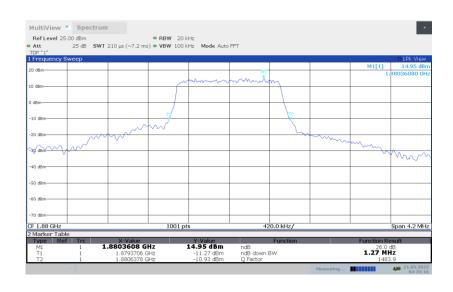
LTE band 2, 1.4MHz Bandwidth, 16QAM (-26dBc BW)
