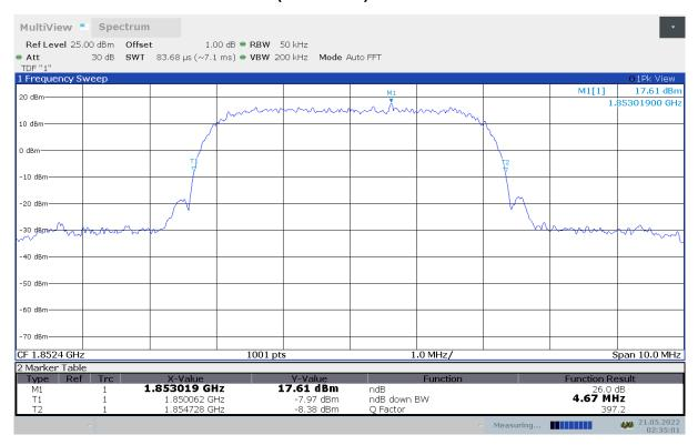
Channel 9400-Emission Bandwidth (-26dBc BW)-16QAM
