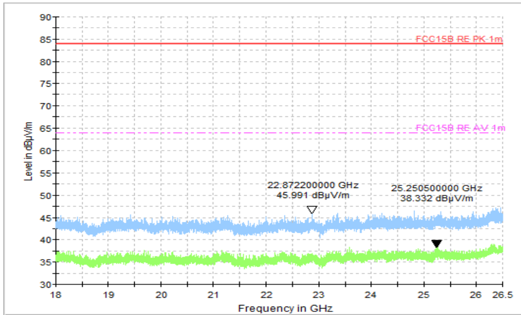
Figure A.1.12. Radiated Emission (LTE receiver Band 5, 18GHz to 26.5GHz)
