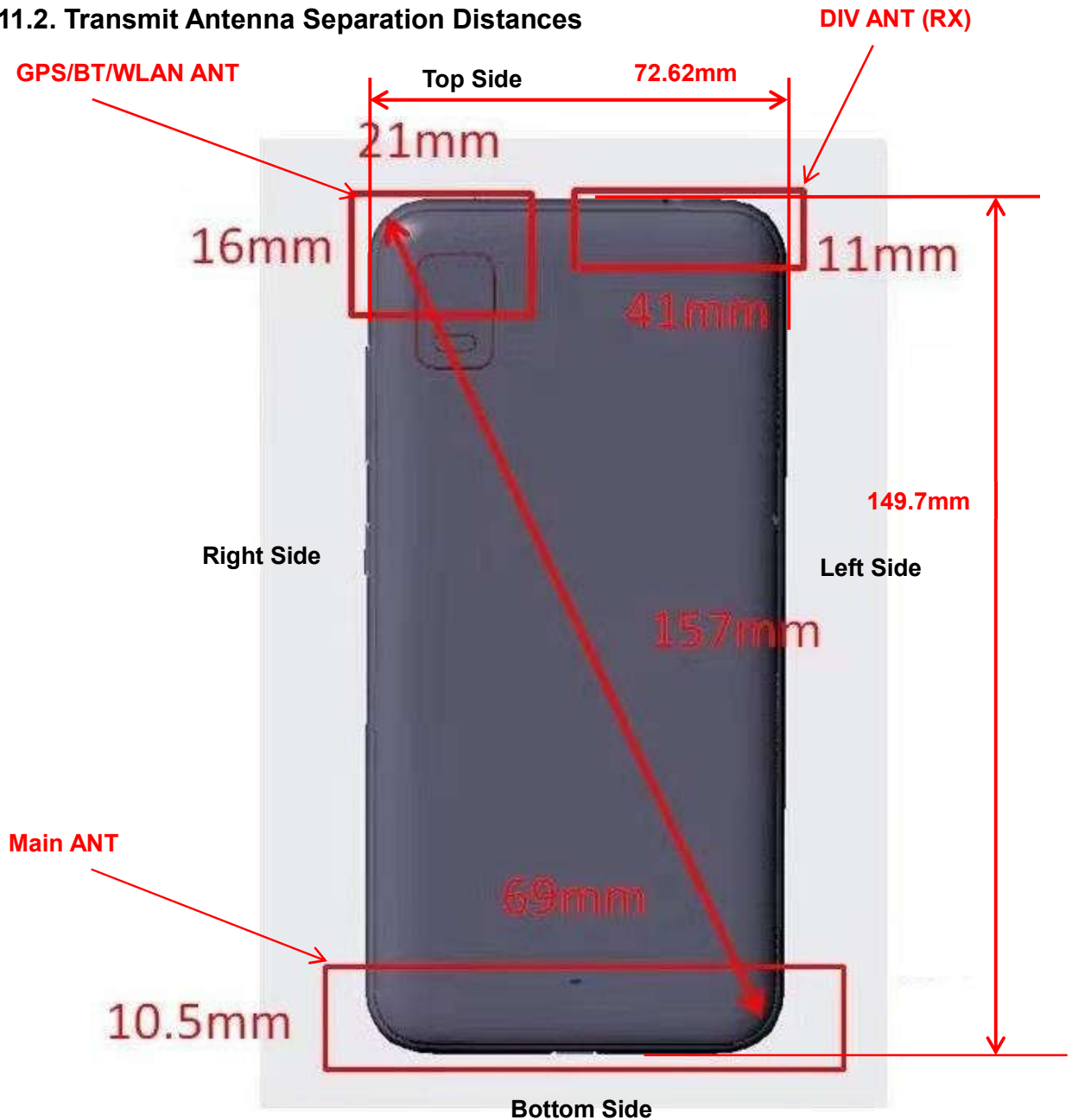
Picture 11.1 Antenna Locations (Back View)
