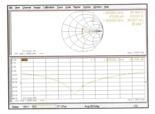
Impedance Measurement Plot for Head TSL
