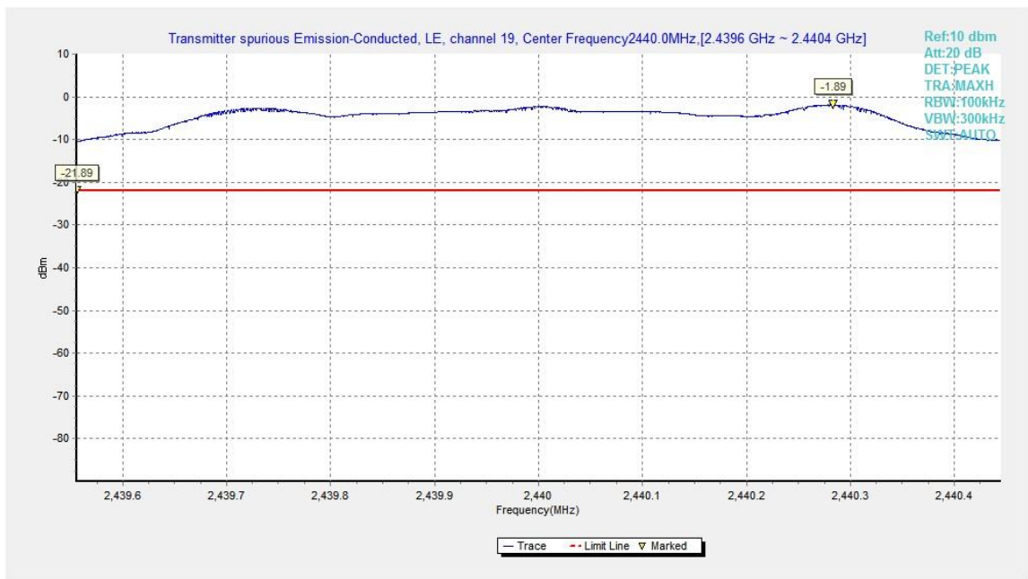
Fig.10. Transmitter Spurious Emission -Conducted: GFSK, 2440MHz
