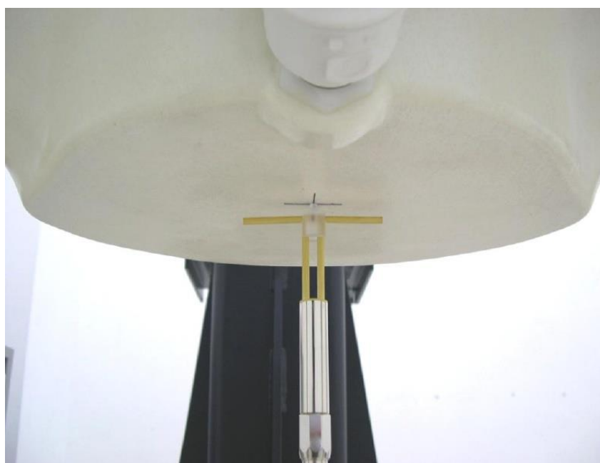
Picture 8.2 Photo of Dipole Setup
