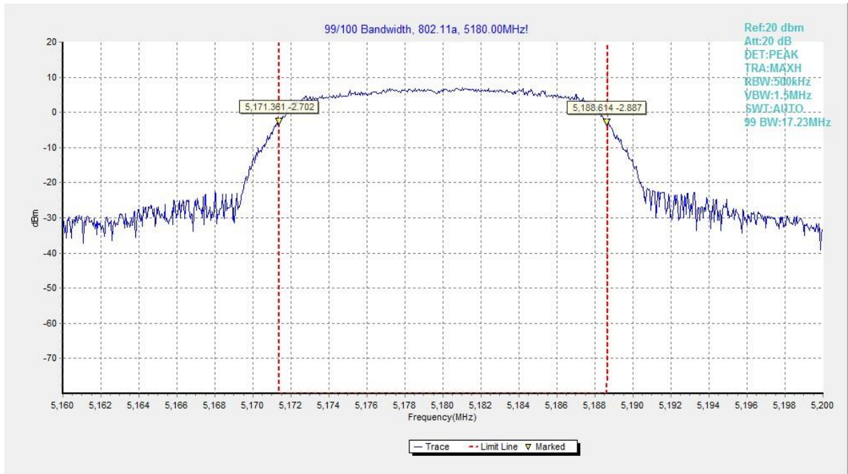
Fig.43 99% Occupied bandwidth (802.11a, 5180MHz)
