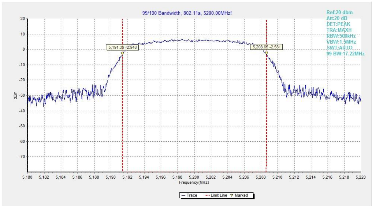
Fig.44 99% Occupied bandwidth (802.11a, 5200MHz)
