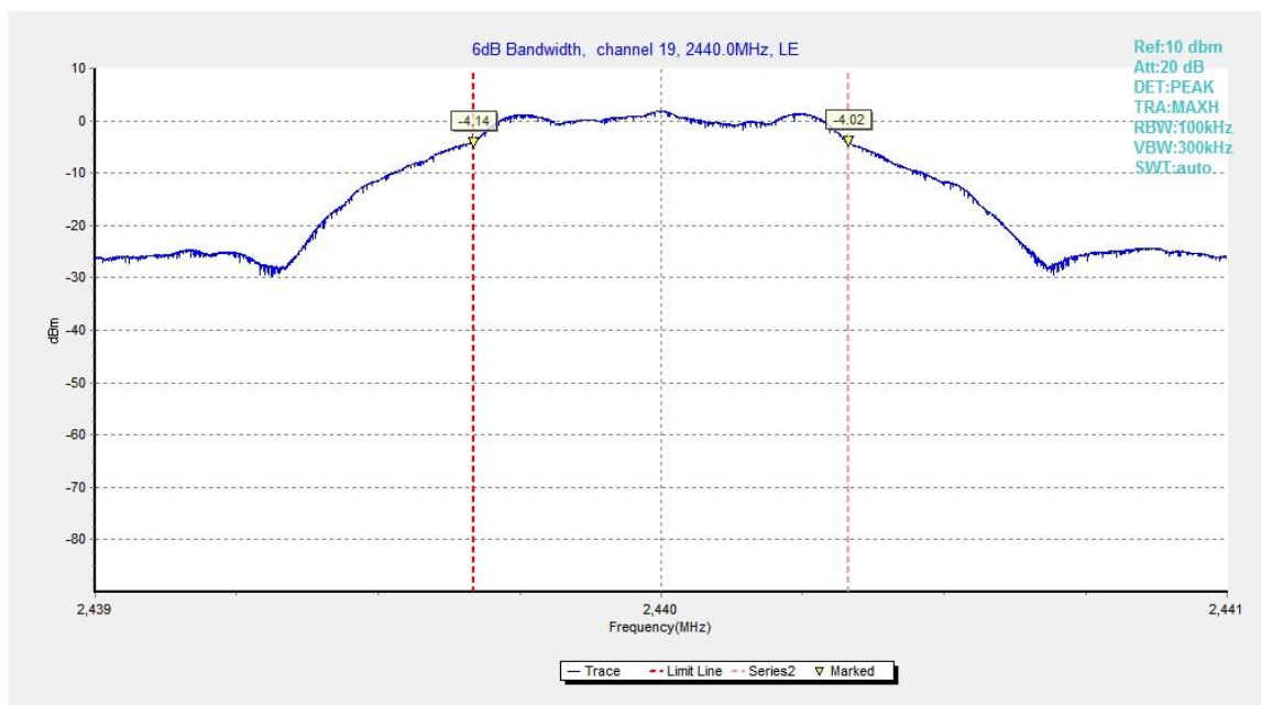
Fig.21. 6dB Bandwidth: GFSK, 2440 MHz
