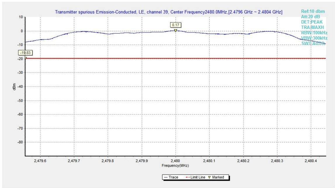
Fig.15. Transmitter Spurious Emission - Conducted: GFSK, 2480 MHz
