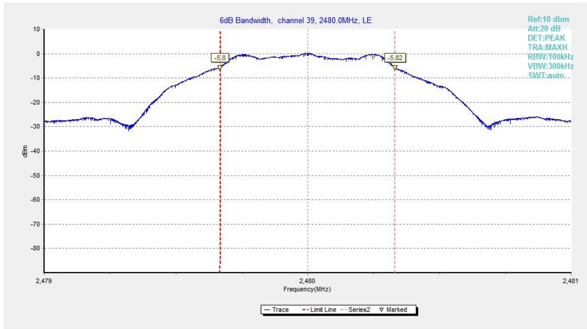
Fig.22. 6dB Bandwidth: GFSK, 2480 MHz
