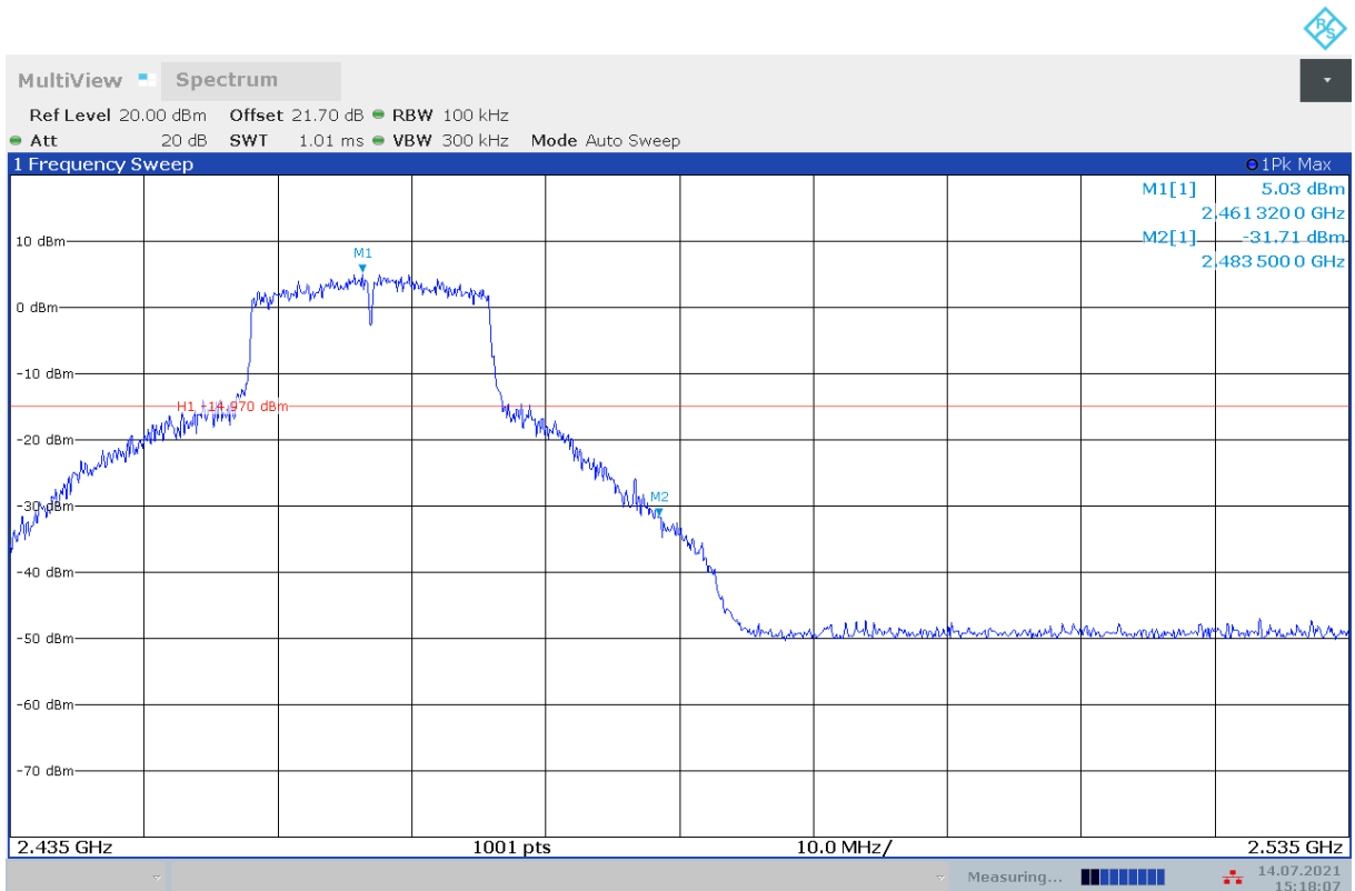
Fig.A.5.6 Band Edges (802.11n-HT20, Ch 11)
